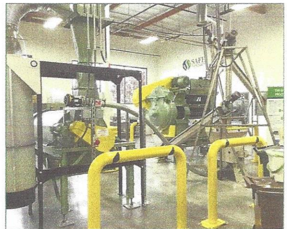
The SAFE extrusion facility in Santa Clara, CA turning food waste into animal feed
