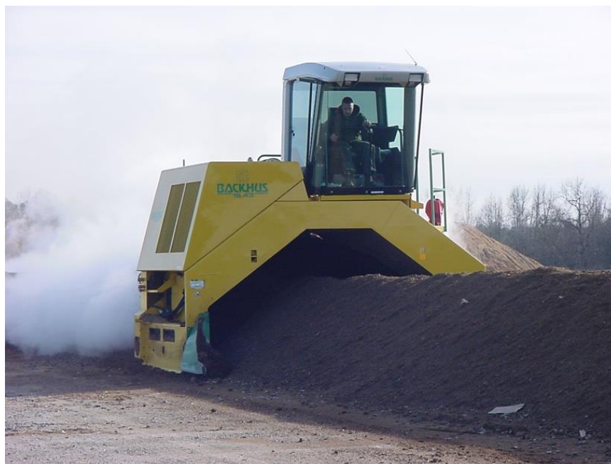
Figure 1. Straddle Windrow Turner Composting
