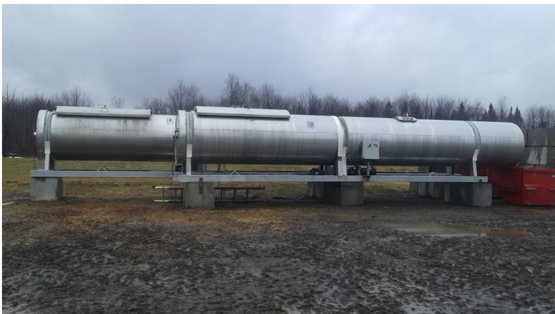
Figure 3. Rotary Drum Composting
